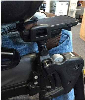
Figure 1: the hardware of the "JourneyCam" device *in situ* on a participant's powered wheelchair.
